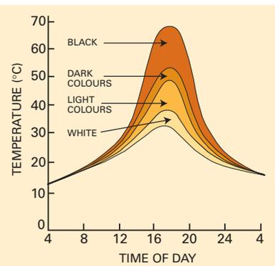
FIGURE 1: Impact of colour on daily temperature of insulated wall surfaces exposed outdoors.
